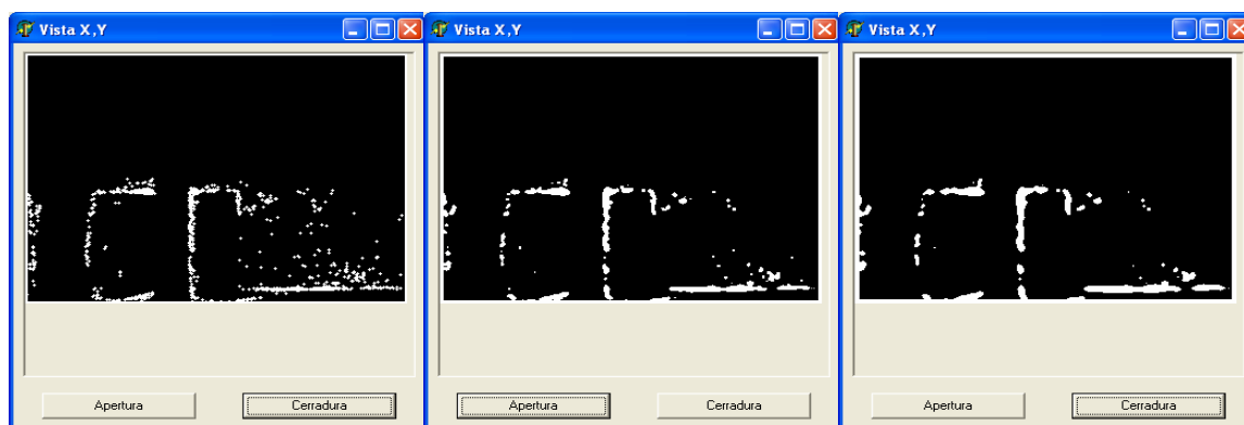
Fig. 16 The X-Y view. We apply the opening operation to deleted isolated flies, next we apply the closing operation to delineate the objects
