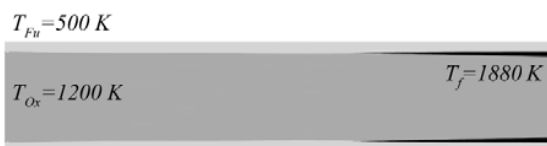
Fig. 4 Flame position in combustion chamber
