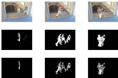
Fig. 10. Background subtraction results. The first row shows input video frames (at Brisbane railway station). Second row shows background subtracted frames. Third row shows the background subtraction result after median filter.
