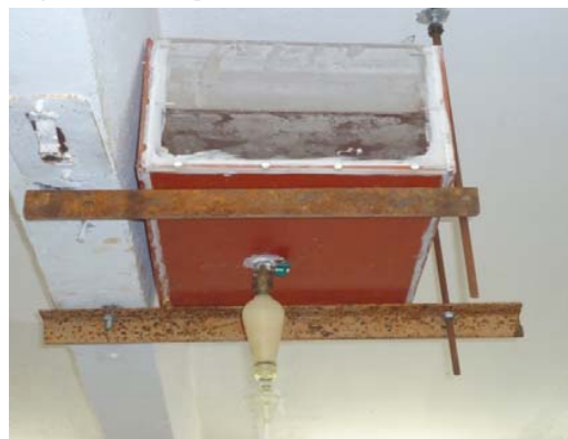
Fig. 2 The water tub, the burette and the capillary tub
