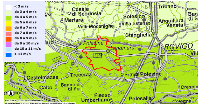
Fig. 6 Average wind speed at 100 m above the ground for the site of Lendinara (from: [12])
