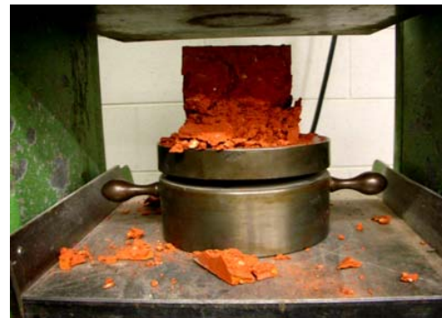
Fig. 6 Compressive strength test
