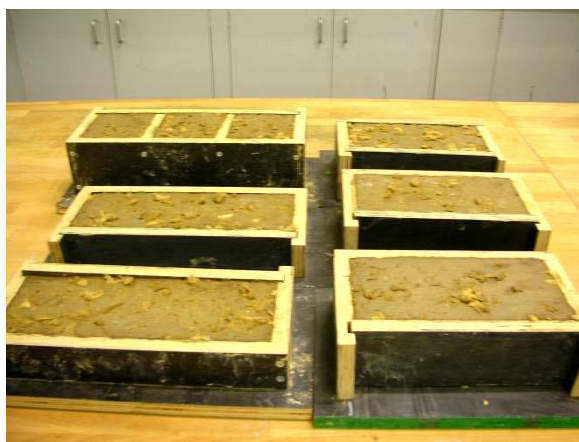
Fig. 2 Compacted bricks, beams and cubes (soil-CBs mix)
