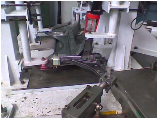
Fig. 1 Cross member, the triangular part and the force inducing machine
