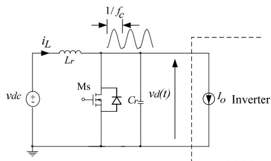
Fig. 1 Resonant dc link equivalent circuit with load  $I_o$
