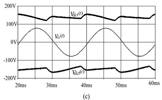
Fig. 7 Simulation results of FFC-SSDM (a) Chopper output voltage  $v_h(t)$  and its harmonic spectrum (b). (c) DC bus voltage source and output voltage
